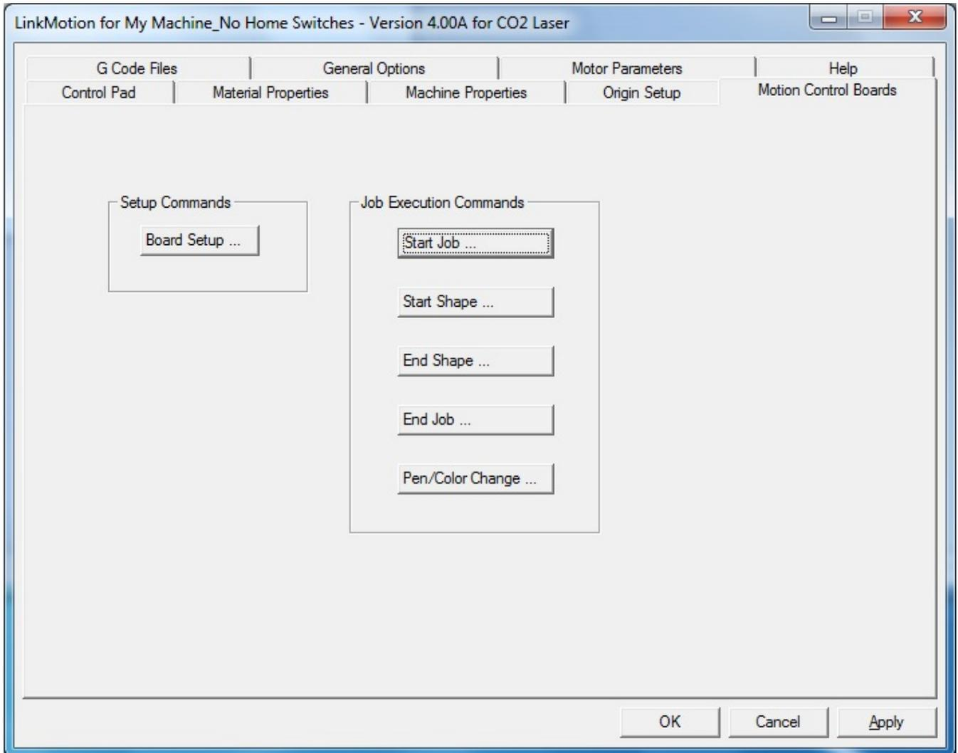
Commands unique to a specific machine can be inserted at the above locations. Many times these are M codes which activate the spindle, vacuum, lubrication, and other functions.
