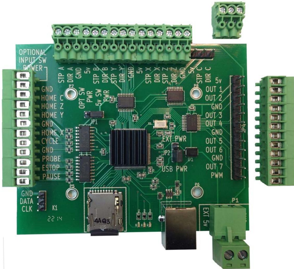
Note that there are two jumpers on the board Jumper to the right of the processor and second onto the left and above the processor.
