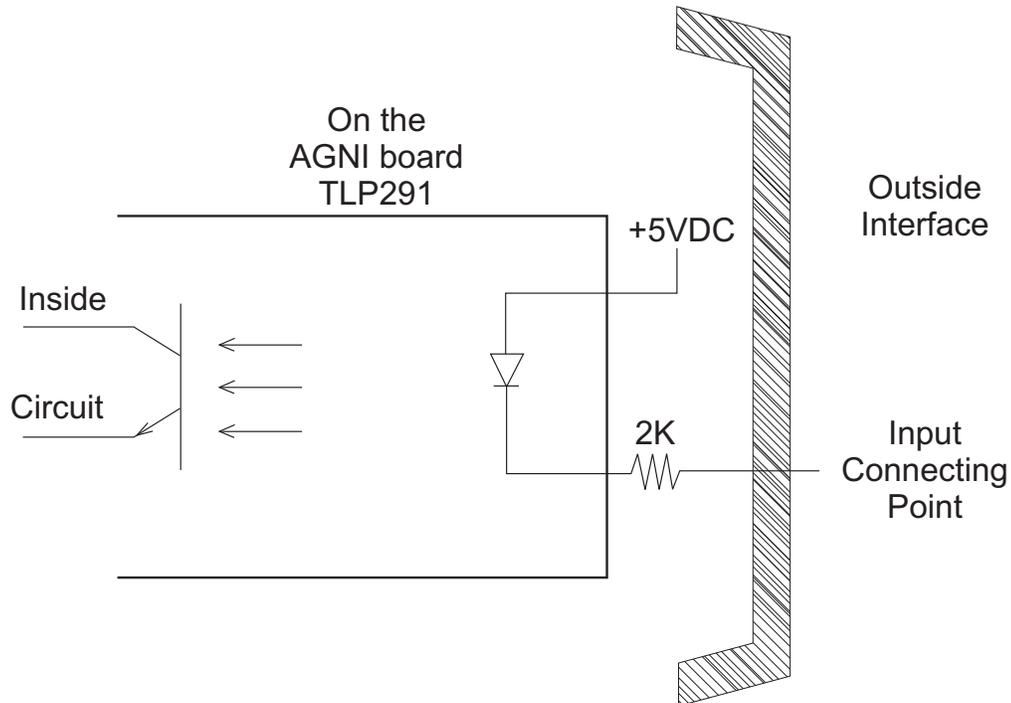
All the inputs are optically isolated with a 2K resistor to limit the current flowing through the diode. Each of the inputs is equipped with the above circuit.
