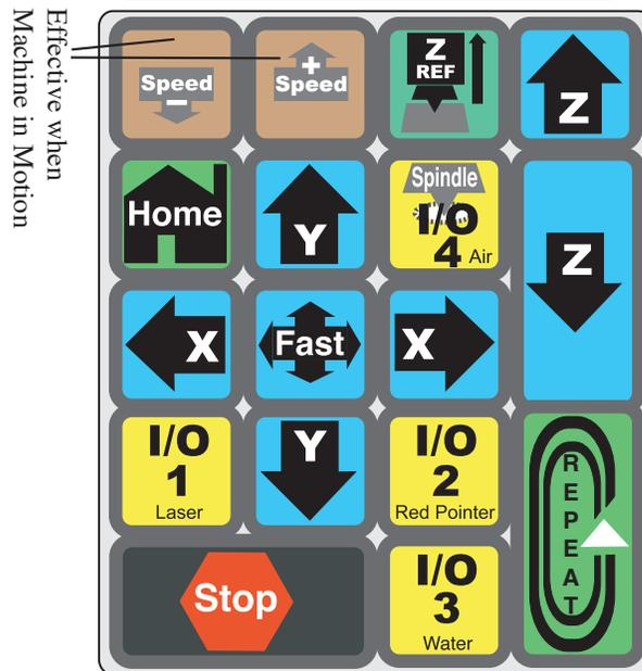
All the keys are active when LinkMotion Control Pad is in foreground on the screen **except the keys for Speed + (Up) and Speed - (down)**. Speed Up and Speed Down keys are effective when job is in process and machine is moving. Speed up key will not go to any higher speed then what you have declared in the Job feed rate of Materials Menu.
