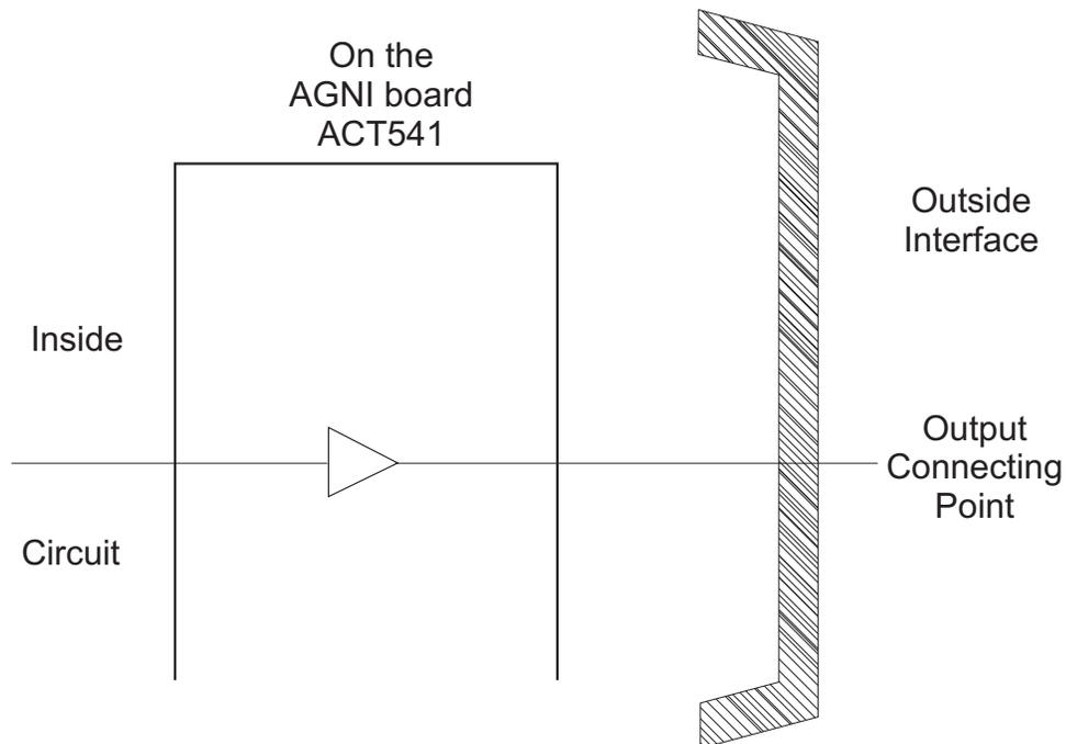
The controller is equipped with output line drivers IC's ACT541. Each line is capable of **sourcing or sinking 20 milliamps**. This makes it very nice to directly connect to step motor drivers. An output can connect directly to a solid state relay for controlling the heavy load.
