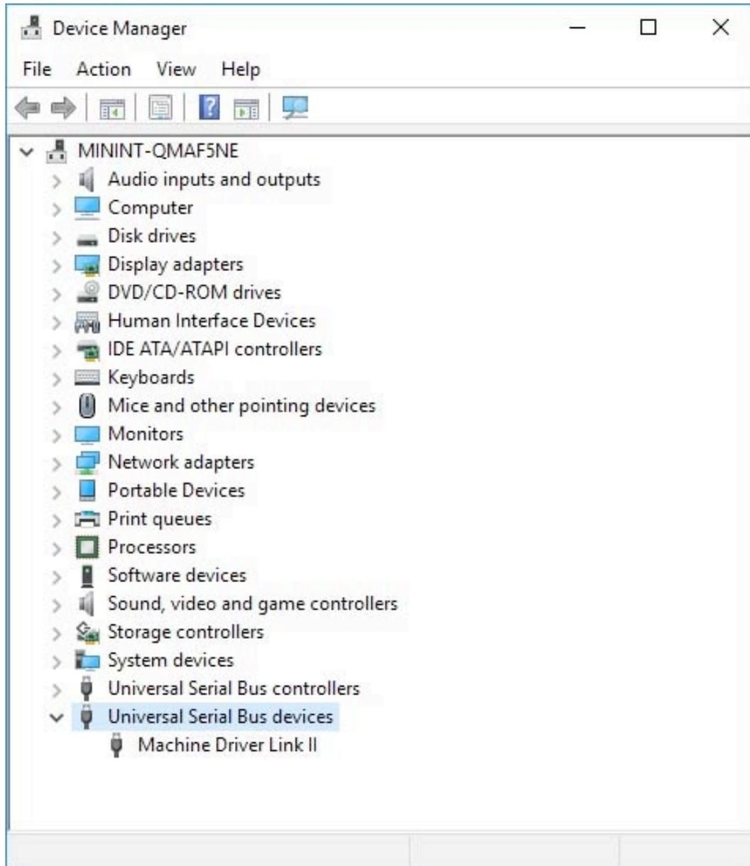
Name of the device once installed will show as “WinUsb Device” and it will show the proper name “Machine Driver Link II” after the restart of the operating system. As long as it is connected properly it will display any one name. **If windows standard USB device driver is not properly installed it will not display this name and will not communicate with new AGNI USB Controller.** Please make sure and install proper driver for USB device.
