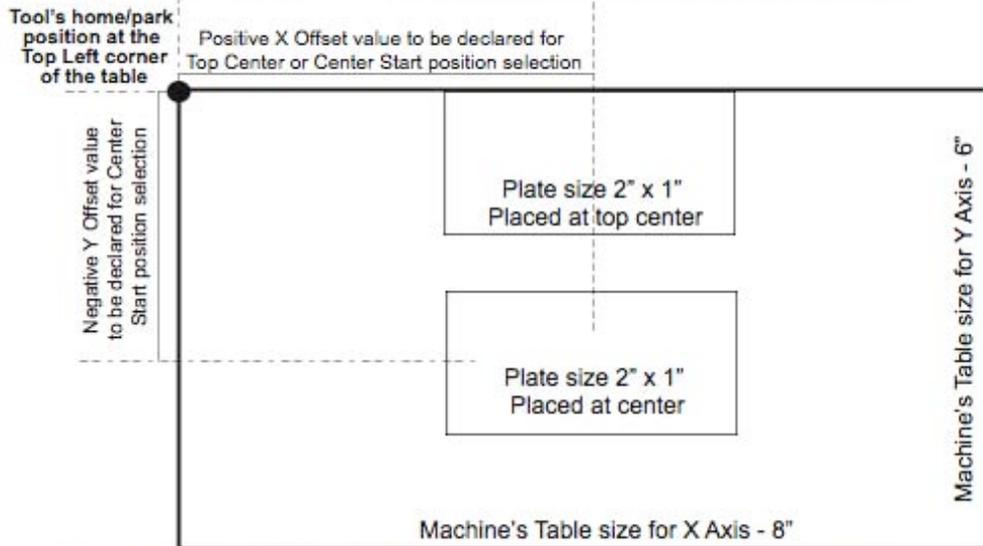
Tool is parked at the Top Left corner of the table(machine) and home position selection should be Top Left. Following three choices are available for Start position and respective offset values to enter:
