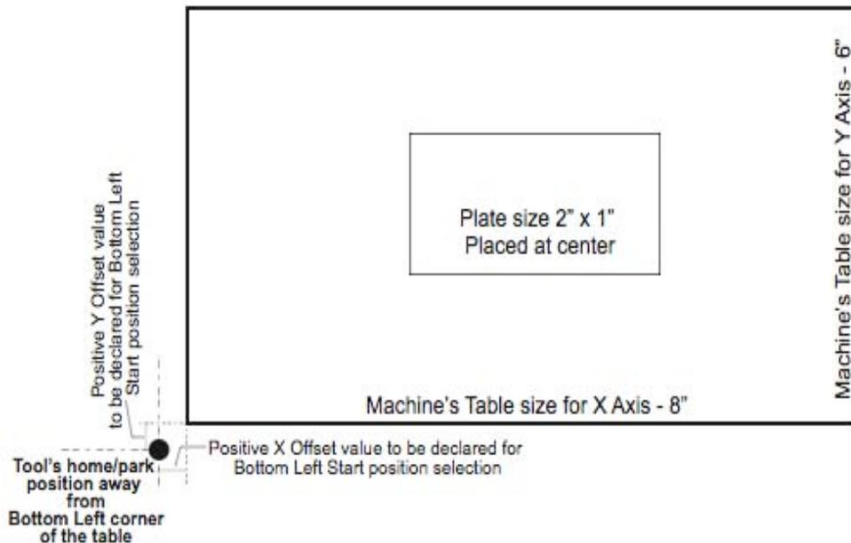
Tool is parked at the Bottom Left and away from the table(machine) and home position should be Bottom Left. Following choice is available for Start position and respective offset values to enter:
