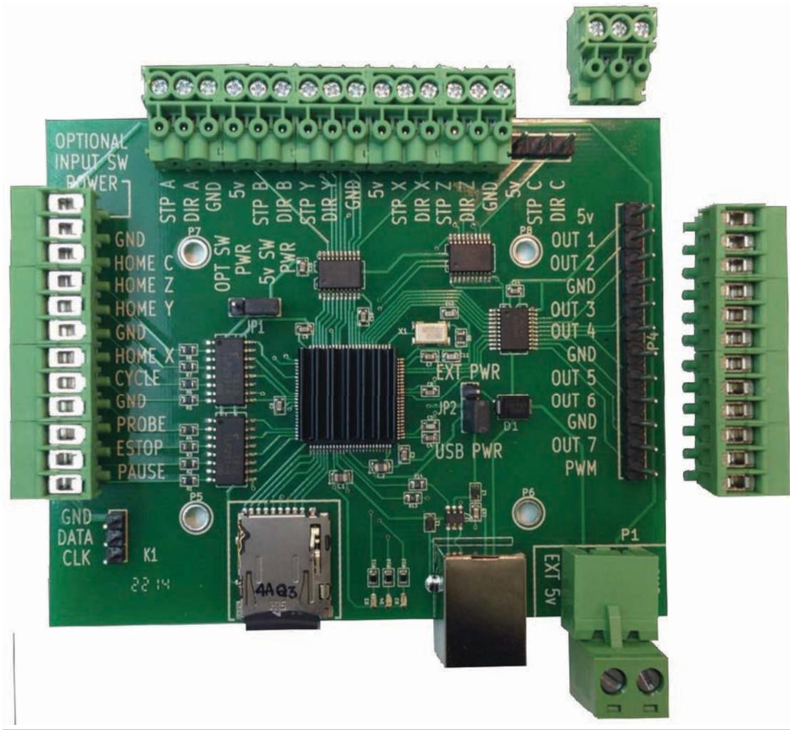
This newest **AGNI-IIP controller** has Phoenix-type connectors that can be plugged in two different ways compared to earlier AGNI II version that had screw terminals. Two different positions are available such that wires can come out either from the sides or from the top. It is slightly smaller in size and all dimensional details are given on the following page. Wiring information is printed on the board and remaining other technical information is provided in the following pages.
