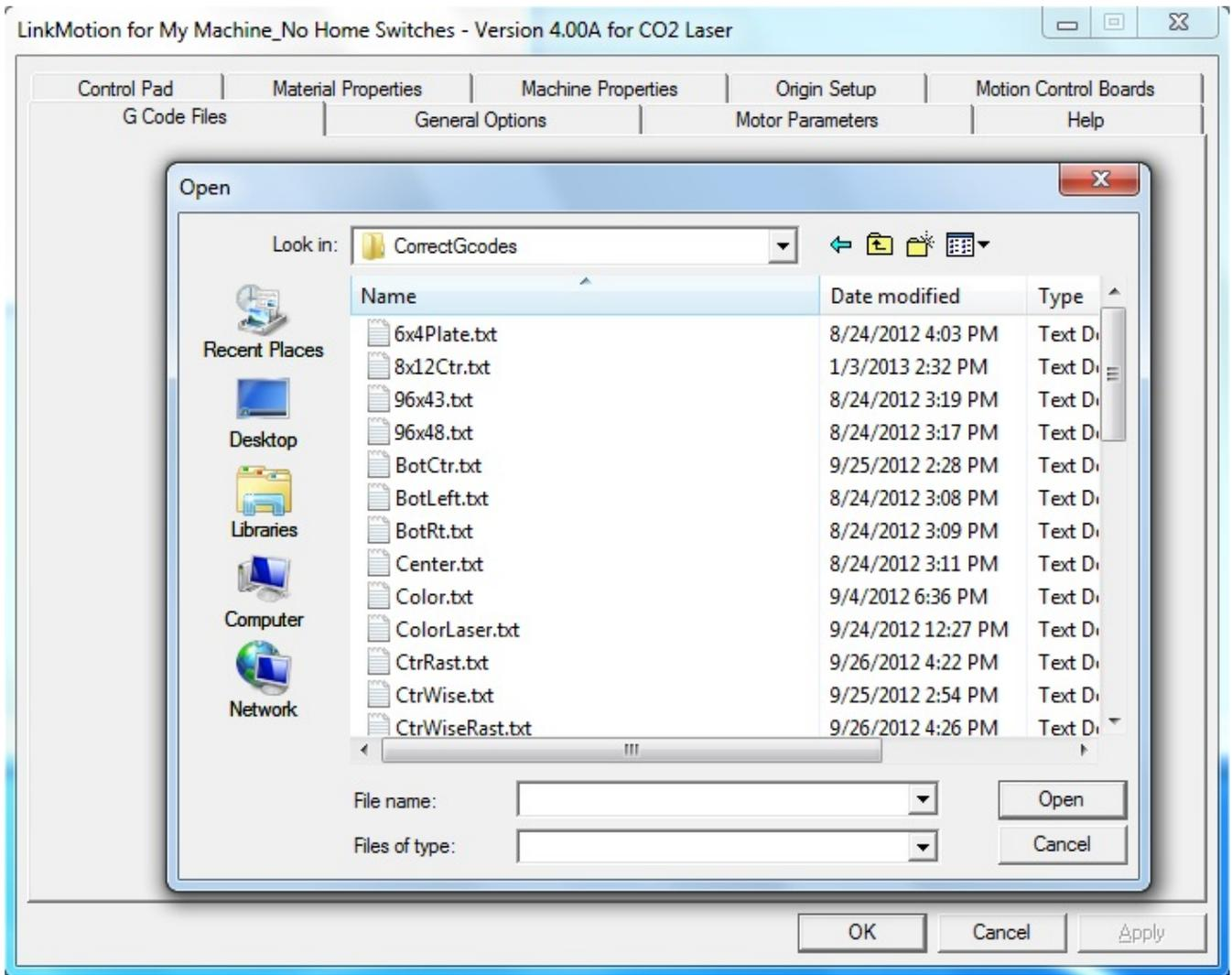
This feature will send previously generated G-Code files from LinkCAM or other CAM programs to CNC machines using the LinkMotion USB driver. Solustan has added custom G codes to handle bit maps and custom M codes to handle frequency and power levels. **The user needs to make sure that you have setup all the parameters for your machine properly by going to the Machine Properties, Material Properties, Motor Parameters, Origin setup and Motion Control Boards before sending the file from here.**
