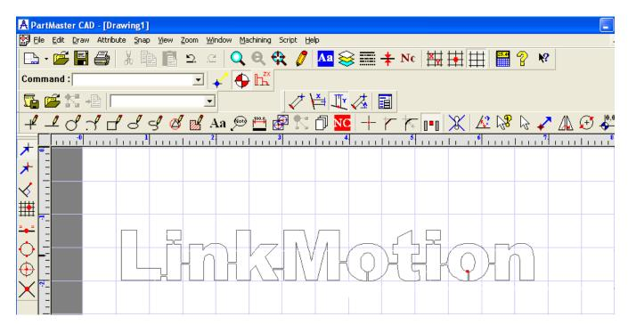
Now it will become **one big connected shape**. Next, **create Contours** using the single shape procedure explained earlier. The job is ready to go to the machine using **Print command**. Select **Contours Only** for output on the machine.
