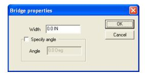
**A bridge properties** dialog box will open. Enter the width of the bridge you want and if you wish to have a bridge at an angle to join some shapes you need to enter the value of that angle here. Click on the OK button.
