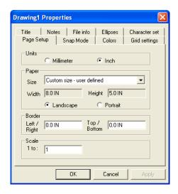
Under Page, Setup makes your selection of units for millimeter or inches.
