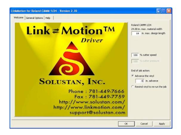
Every cutter has physical limit to the maximum width of material it can handle. However, the length of the design can vary. An appropriate number would be the length the material that can be tracked successfully by the machine. Anytime you make this change in the value for the length you need to make sure to launch design application like Corel after the change is effective in LinkMotion driver.
