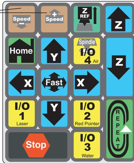
All the keys are active when LinkMotion Control Pad is in foreground on the screen **except the keys for Speed + (Up) and Speed - (down)**. Speed Up and Speed Down keys are effective when job is in process and machine is moving. Speed up key will not go to any higher speed then what you have declared in the Job feed rate of Materials Menu.
