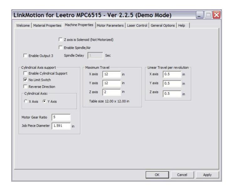
**Z** axis can be selected as motorized or air controlled. For Leetro implementation, it should always be checked. The Leetro controller handles the movement of the Z axis step motor.
