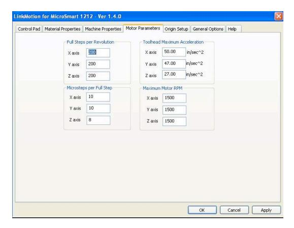
Above values are determined by the motor manufacturer. Enter **Full steps per revolution** values for each axis depending upon the motor and the lead screw size specifications.
