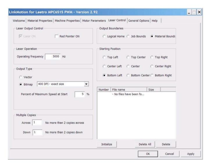
This is the most important part of the settings and selections in LinkMotion for proper output from your lasers system. LinkMotion is a printer type driver and user will spend most of the time designing a job in his/her favorite application program. However, settings and selections here prepare the laser machine for proper output in the intended location on the laser machine.
