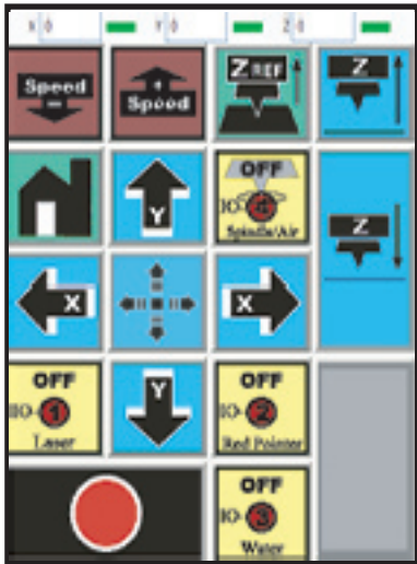
Control Pad on the Keyboard for direct machine control
